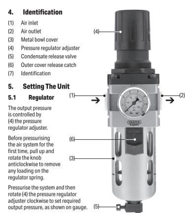
When the required pressure is achieved push in (4) the pressure regulator adjuster to prevent inadvertent adjustment.
